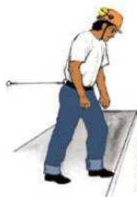
This is an example of a fall restraint system. Fall restraint systems prevent workers from falling.
