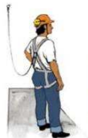
This is an example of a fall arrest system. Fall arrest systems protect workers after they fall by stopping the fall before they hit the surface below.
