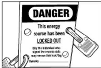
Figure 3: Example of multiple locks on a lockout tag
